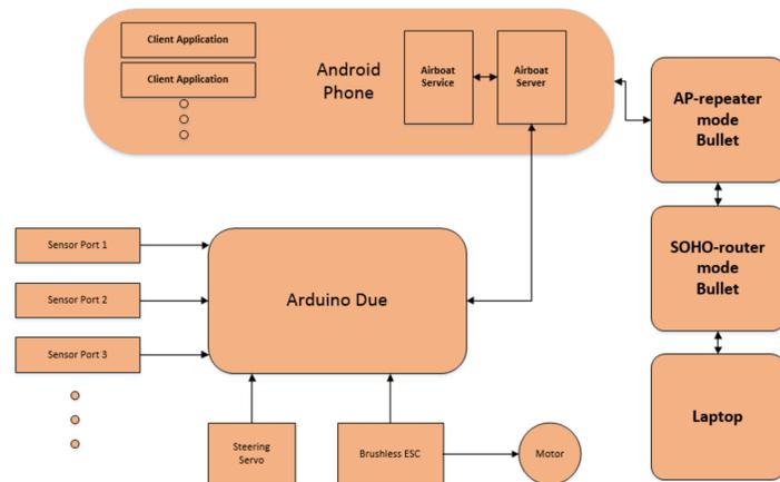
We are working with a team of robotic boats, a human operator gives high level commands to from the shoreline. The setup earlier used a single Bullet router which was put on the shoreline, but had decreased range talking to the boats due to the effects of water on electromagnetic waves. By configuring another Bullet in AP-repeater mode and putting it on a boat, we can extend the range of the network.
