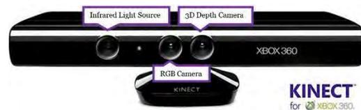
Figure 1: Kinect 360 and its components
