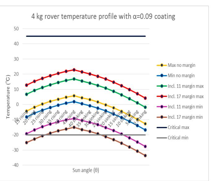
A lunar rovers temperature is inversely proportional to its surface area. Smaller rovers have a much harder time cooling down.
