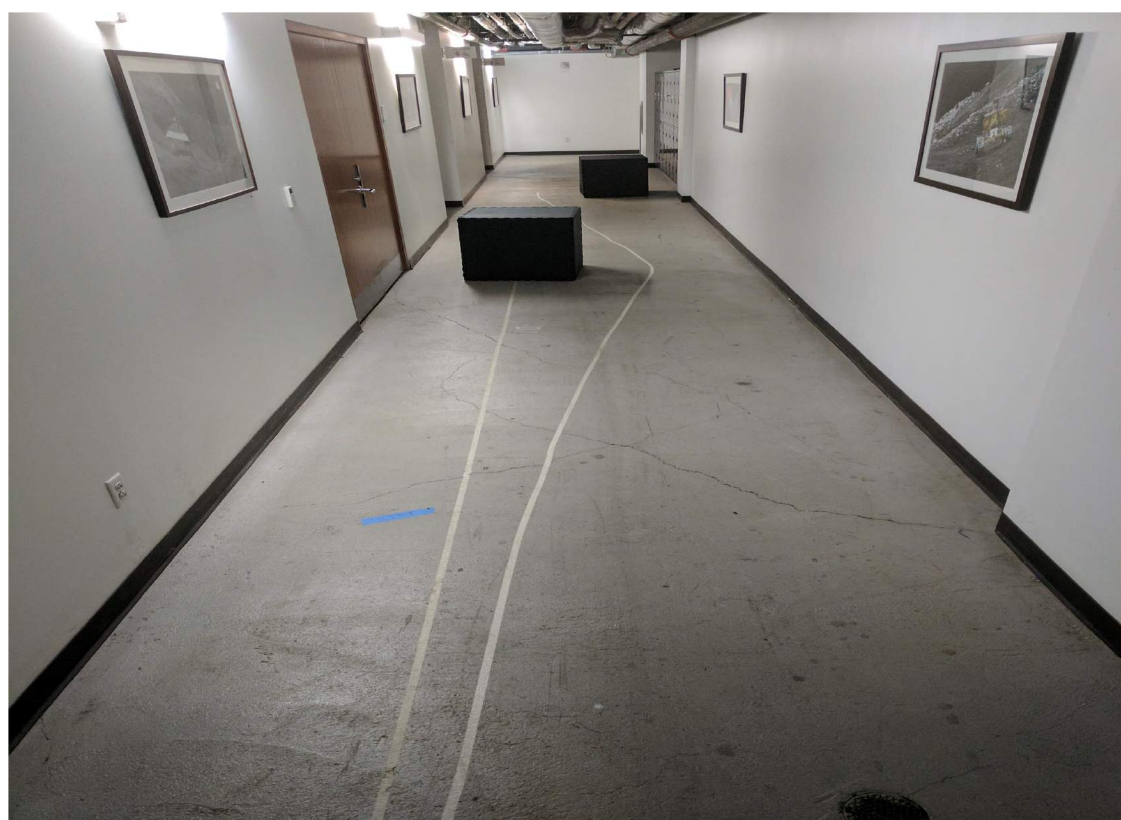
Test environment used for ground robot teleoperation tests. The user navigates the robot around the black obstacles. The white line on the ground is provided as a reference.
