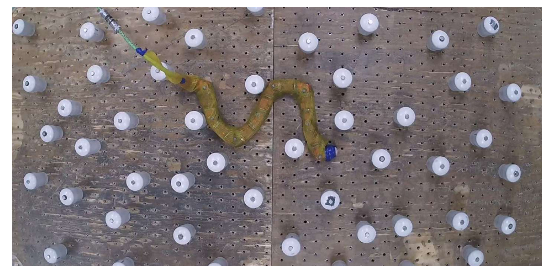
Figure 5: Snake robot wearing a polyester sleeve traversing an unstructured peg array.
