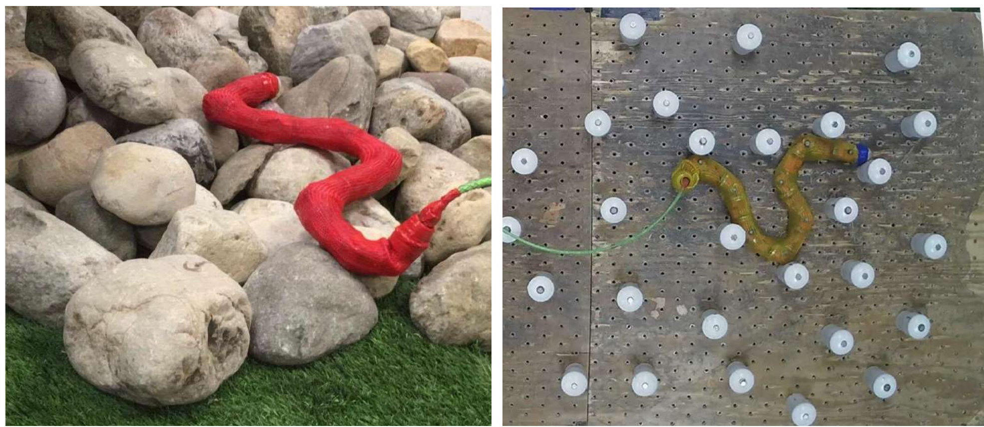
Figure 1: Snake robot in unstructured environments we present a learning approach that leverages recent advances in distributed reinforcement learning to learn a decentralized control policy.
