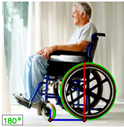
Figure 6: This is the result of the implemented algorithm where one big and one small wheel are detected and the orientation is estimated. Also, the ground points are marked at the bottom of the detected wheels.
