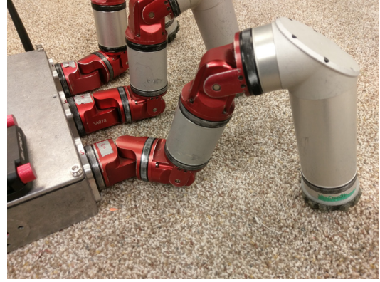
Fig. 1: Hexapod leg joint configuration.
