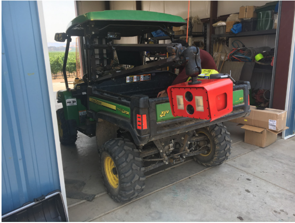
(a) The stereo camera mounted on the back of a field utility vehicle
