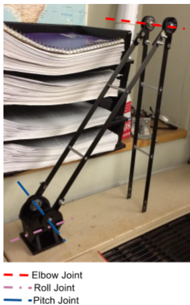
Fig. 2. Physical model of the manipulator with joints labeled
