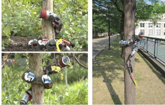
Fig. 1 Snake following a helical trajectory when climbing poles
