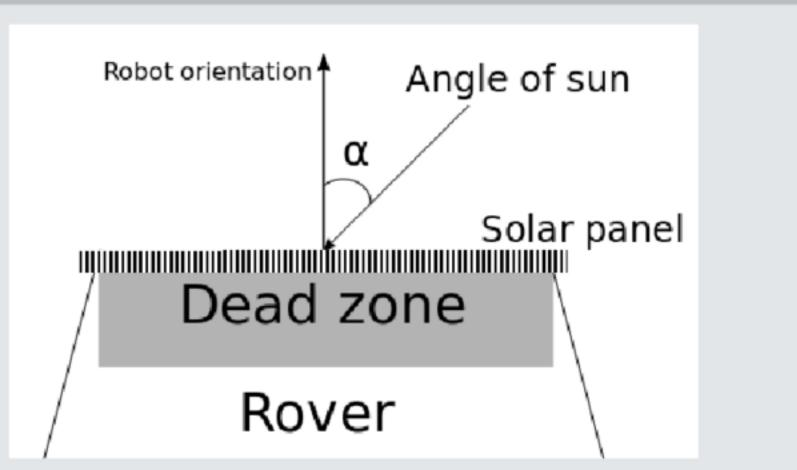
panel solar and angle between the factor and the panel normal  $\alpha$ ,  $p_{solar} = \eta \cos \alpha A$
