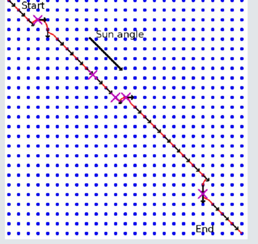
The planner running on a map of lunar terrain at The rover turns off its motors to decrease internal heat generation and reduce its temperature. The X's represent where the rover stops.
