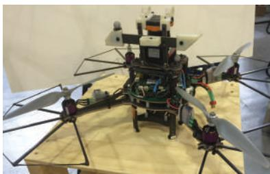
Fig.1 A quadrotor testbed with sensors
