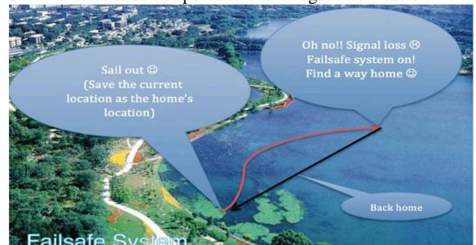
Fig. 7 Failsafe System mechanism
