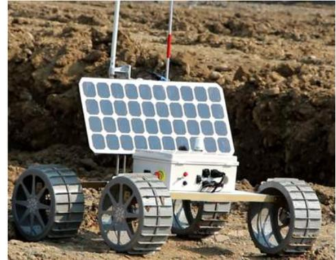
Fig. 1. Andy 2 rover exploring a simulated lunar pit in the Robot City test site. The Andy rover mission aims to explore the Lacus Mortis pits on the Moon as part of the Google Lunar X-Prize.
