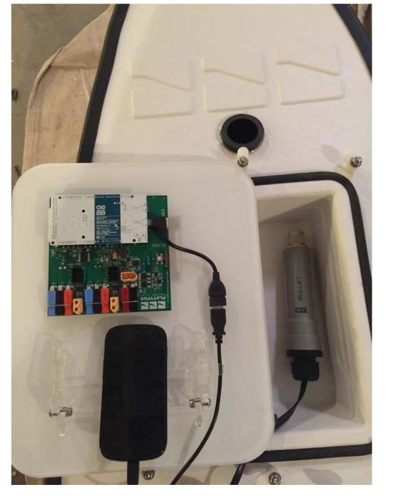
Now we put the Bullet in the boat, which talks to the boat's phone(Also a sharkfin antenna connect to the Bullet), which is connected to Arduino Due. The laptop GUI will send the navigation
