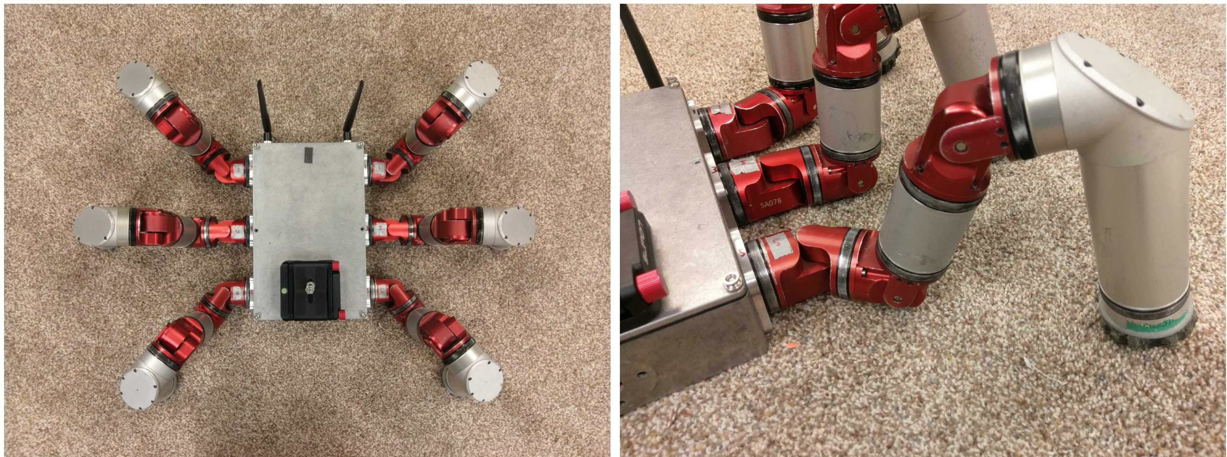
Figure 3: Experimental Platform: modular, series-elastic hexapod robot aerial view (left); hexapod robot leg joint configuration (right).
