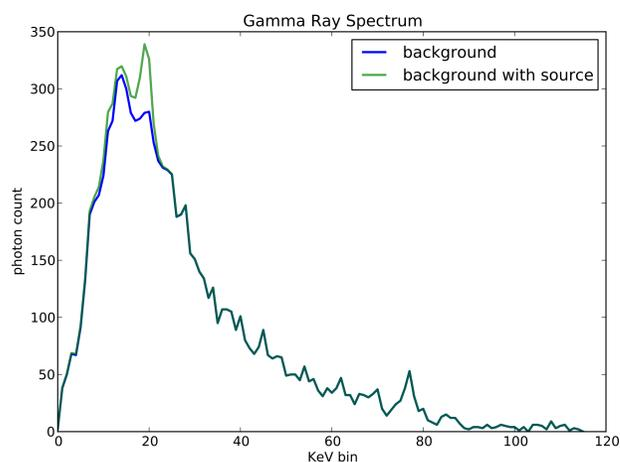
A typical spectroscopic measurement, with and without source injected.
