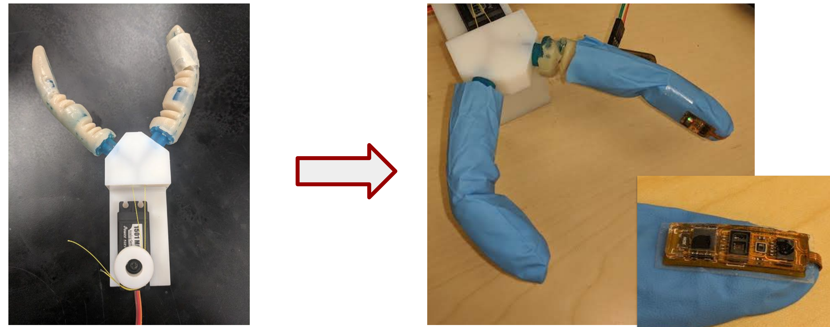
Figure 3. Nitrile gloves were used to aid the adhesion of the tactile sensor to the fingers of the anthropomorphic two-finger gripper.
