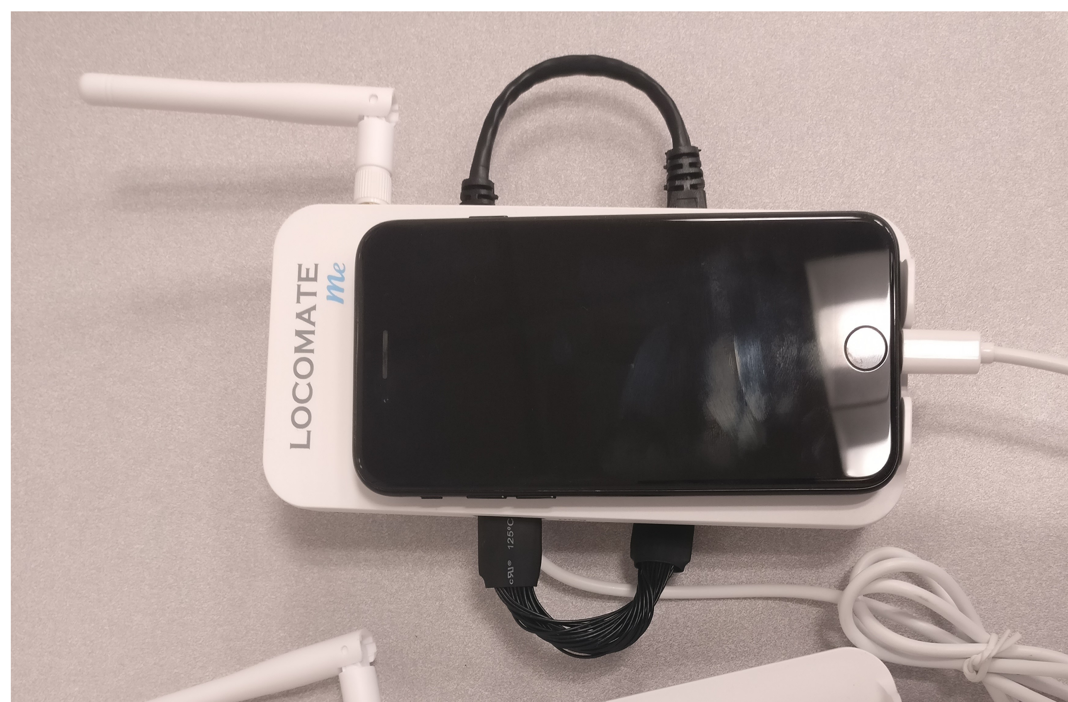
DSRC Sleeve with iPhone 7 used for testing
