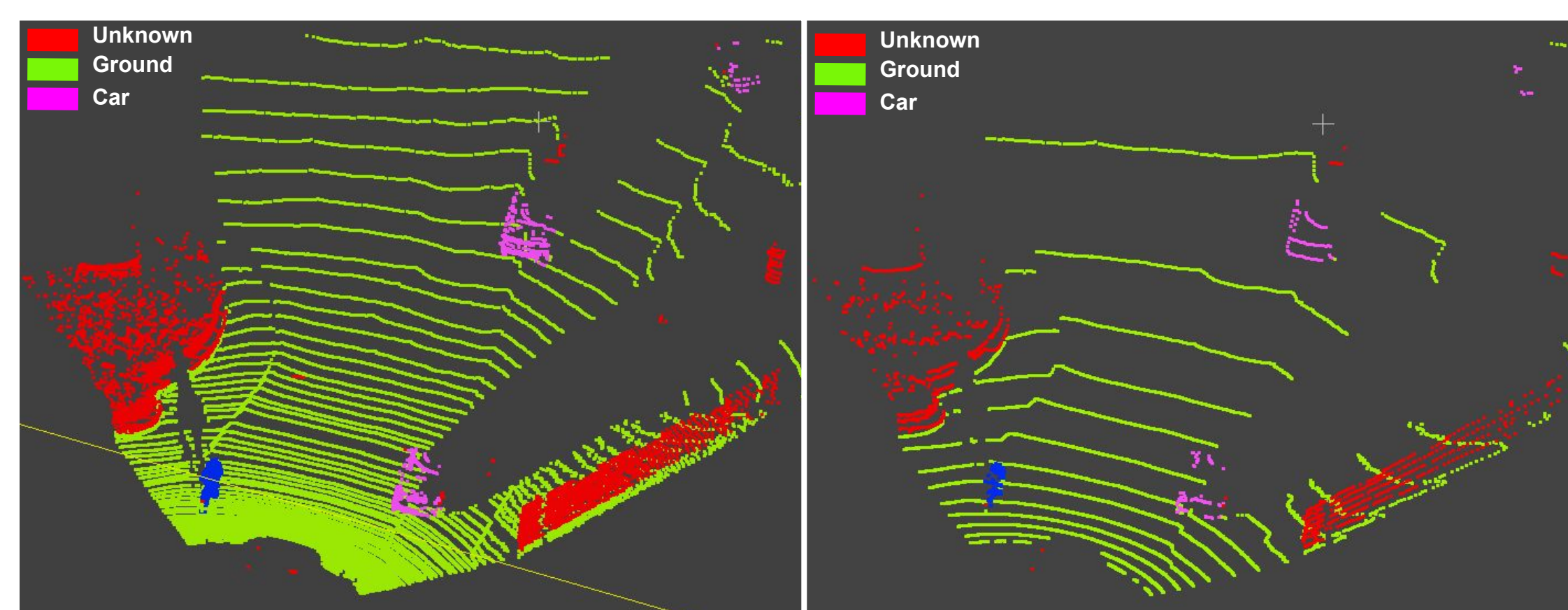
Fig. 2: Original 64-ring LIDAR scan (left) vs down-sampled 16-ring scan (right)
