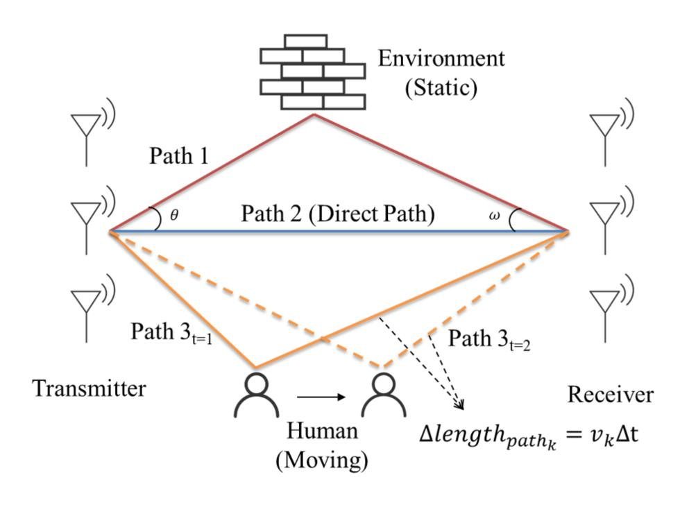
CSI characterizes how wireless signals propagate from the transmitter to the receiver at certain carrier frequencies.
