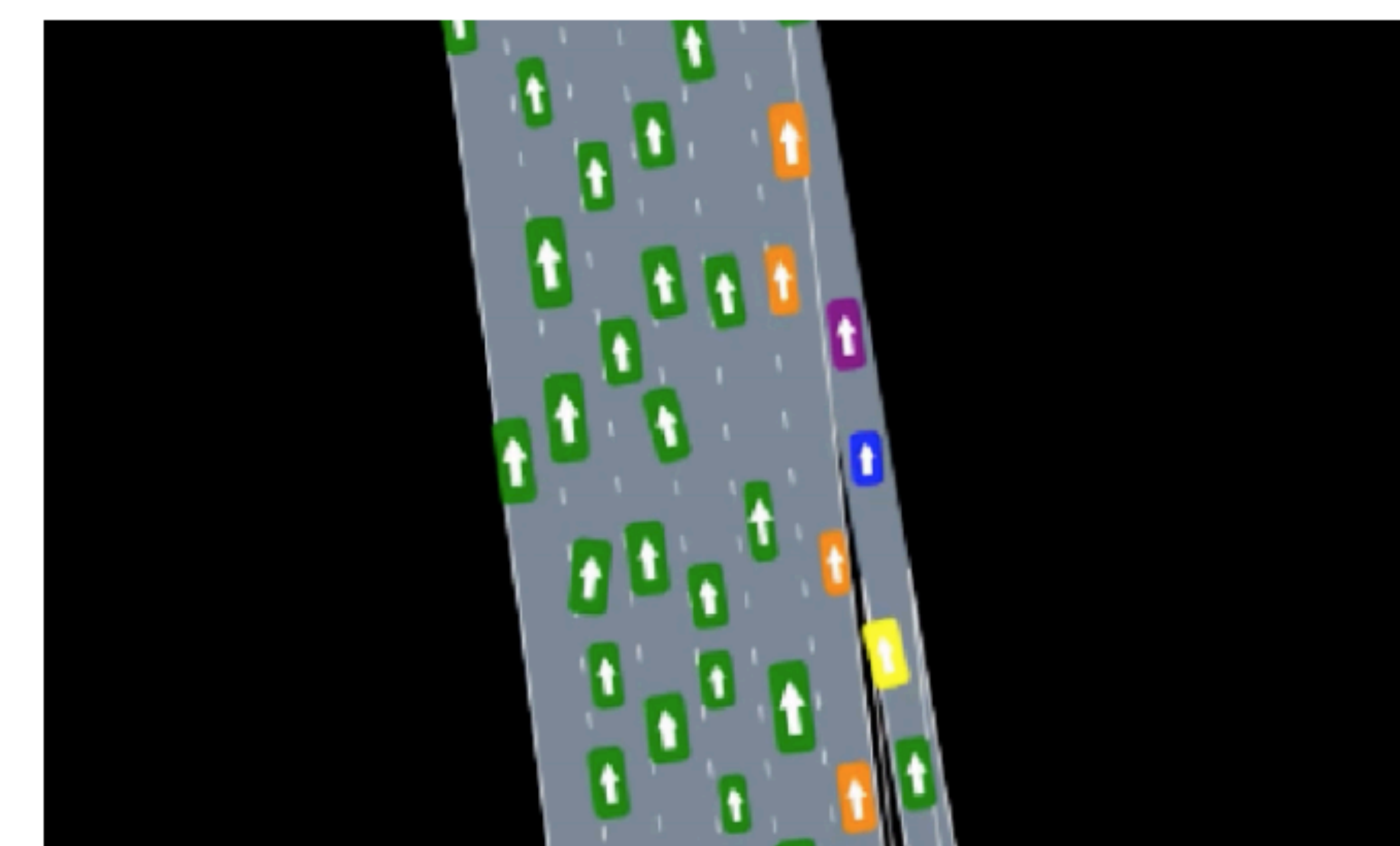
Fig. 3. Diagram of the vehicles that the ego-vehicle has access to - two in the merging lane and four in the host lane. The ego-vehicle is in blue, the merging neighbors are in yellow, and the host neighbors are in orange. The leading vehicle that IDM is distance-keeping to is in purple. Green vehicles are unobserved by the ego-vehicle.
